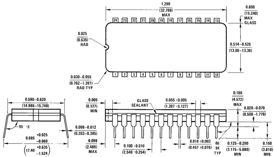
**24-Lead Ceramic Dual-In-Line Package (J)**
