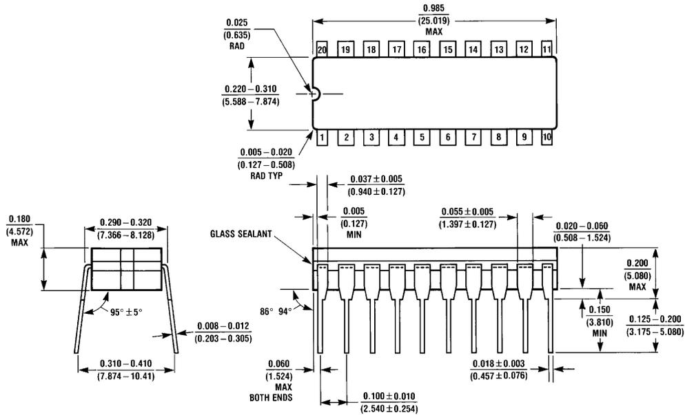
**20-Lead Ceramic Dual-In-Line Package (J)**
