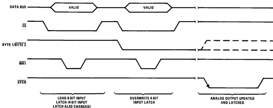
$\overline{\text{WR2}}$  tied to a logic low (0V)
