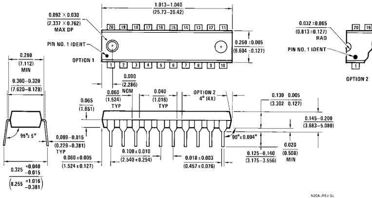
**20-Lead Molded Dual-In-Line Package (N)**
